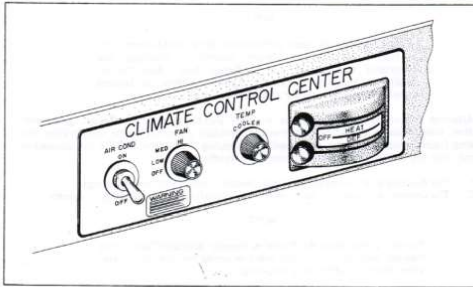
Air Conditioner Controls
